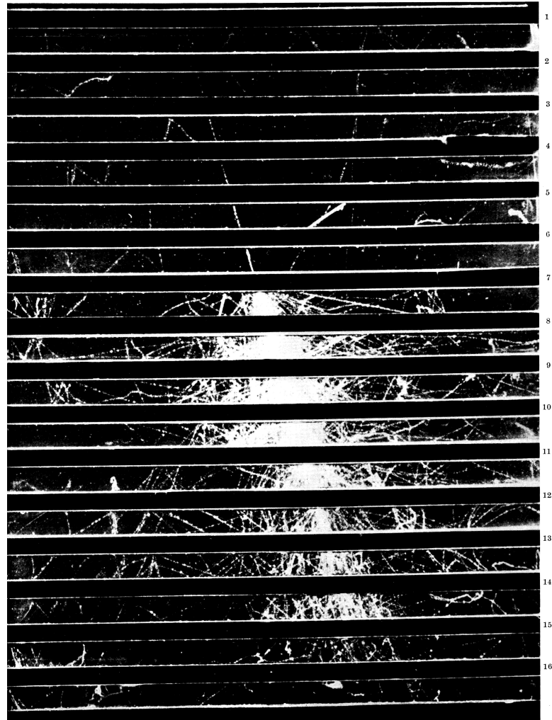
Figure 2 : Image of a particle cascade, or shower, as seen in a cloud chamber at 3027 m altitude. The primary particle is estimated to be a proton of about 10 GeV. The first interaction would most likely have been in one of the lead plates. Neutral pions feed the cascade which multiplies in the lead. Charged pions make similar interactions to protons, or decay into muons. The cross-sectional area of the cloud chamber is 0.5 \times 0.3 \text{ m}^2 and the lead absorbers have a thickness of 13 mm each [8].
